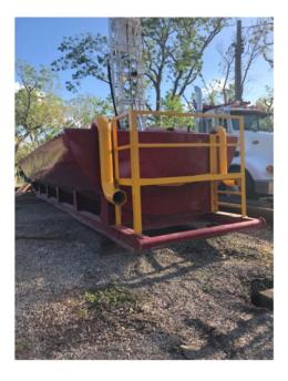
Figure 2: Frac Tank—Used to Collect and Stabilize Acid From the Well
